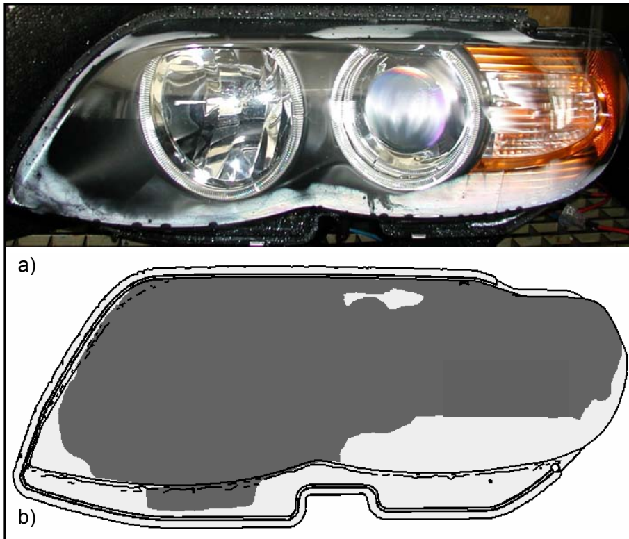
Fig. 7: Condensation zones a) experimentally produced and b) forecast by simulation.
