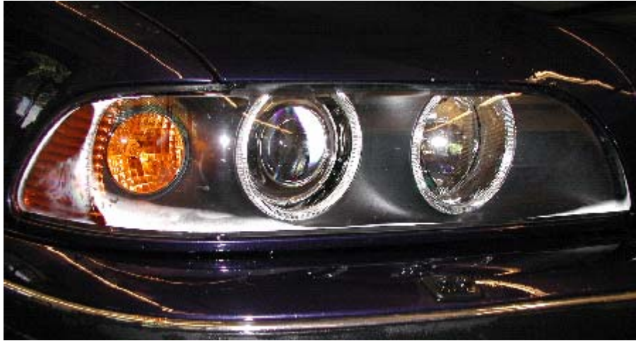
Fig. 5: Headlamp with condensation (light-coloured areas on the PCL)
